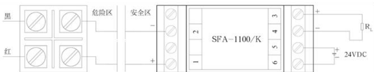
Figure 24 Connection between flow meter and isolated safety barrier
