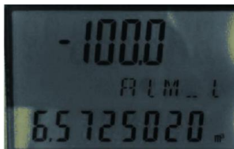
Figure 9 state of modifying the lower limit of the alarm
